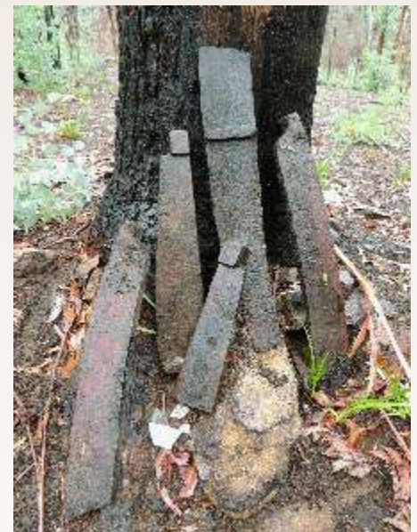
Boiler fire grates from a steam or traction engine
